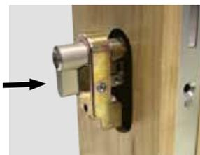
3. Remove the thumb turn from the cylinder by pushing in the release pin on the thumb turn or by using an allen key where appropriate. Next, install the cylinder into the lock in the door leaf from the external side.
